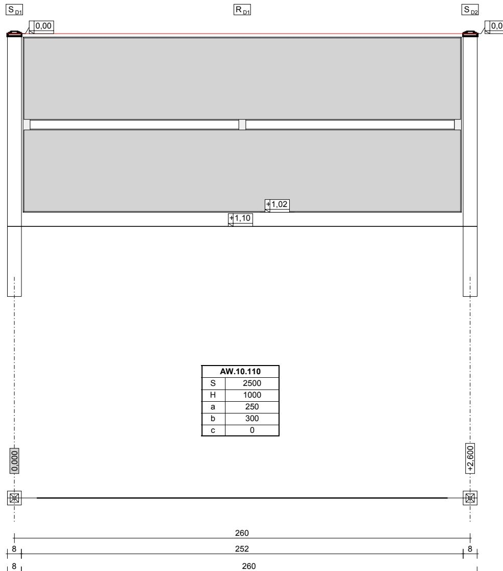
LEGEND:  $S(So)$  – element width [mm];  $H$  – element height [mm];  $a$  – upper crossbar position (for WP and Wk taken together with the arch) [mm];
