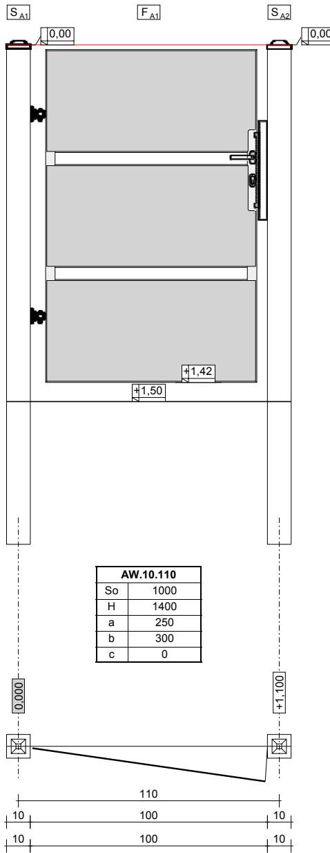
LEGEND: S(So) – element width [mm]; H – element height [mm]; a – upper crossbar position (for WP and Wk taken together with the arch) [mm]; b – lower crossbar position [mm]; c – arch height [mm]
