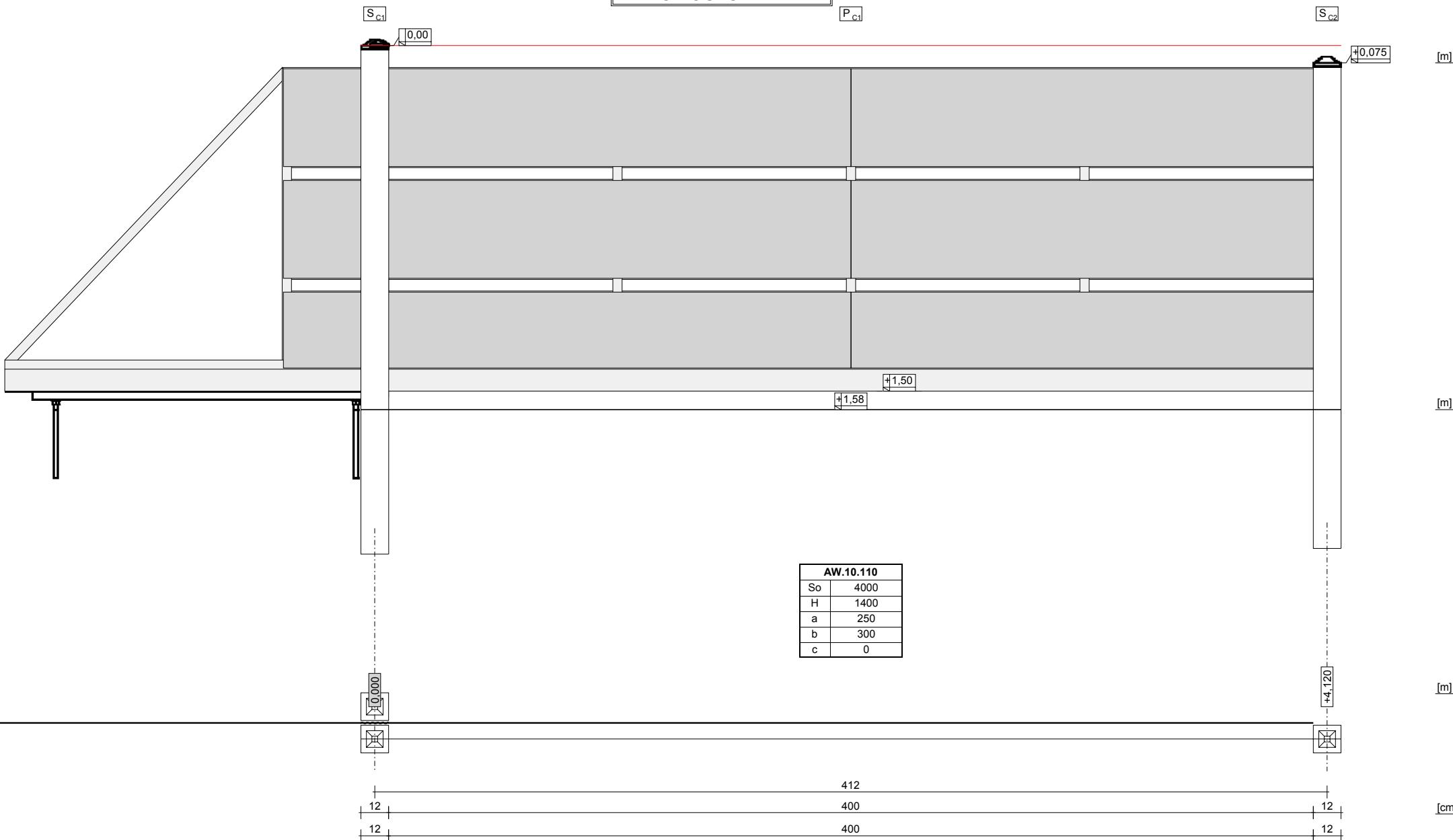
LEGEND: S(So) – element width [mm]; H – element height [mm]; a – upper crossbar position (for WP and Wk taken together with the arch) [mm];
